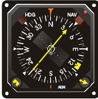
Fig. 4-7. Horizontal Situation Indicator
